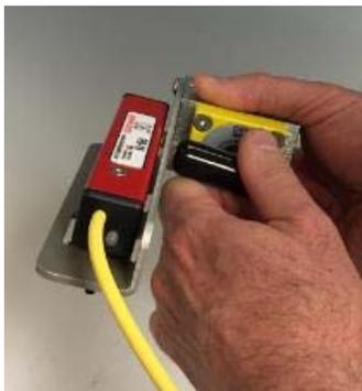
**STEP 2** – Determine which slots that the plunger should be in for your application and adjust plunger to those slots. Also, determine the starting height of the plunger and tightened the thumbscrews.
