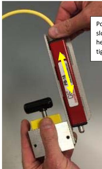
**STEP 3** – Connect the cable to the hand-held controller and the other end to the PB-16 actuator.
