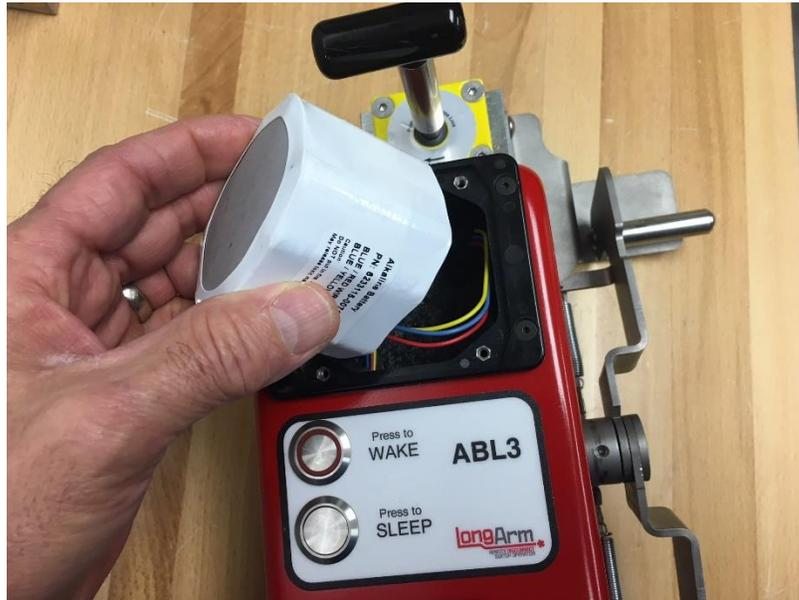
**STEP 3** – Disconnect battery at connector.
