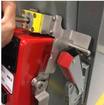
**STEP 3** – With actuator now flush against the MCC door, twist both magnet levers one-half turn clockwise to latch the magnet and actuator in place.
