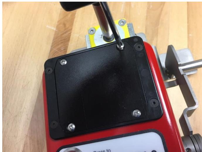
**STEP 2** – Remove battery cover plate and slide battery out.
