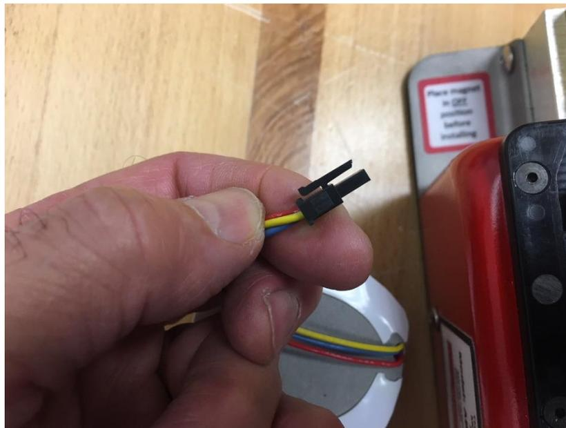
**STEP 4** – Plug new battery into the connector and slide battery into place. NOTE: The battery will only go in one way. The end where the battery leads exit the battery must go in first.
